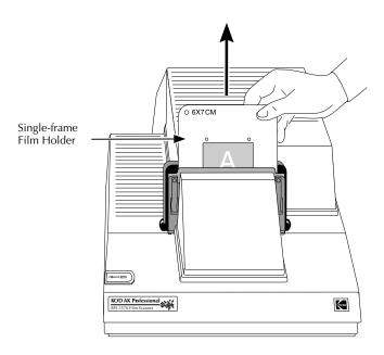
C. If the single-frame holder adapter is not in the Scanner, put it in place in the Scanner. Do so by holding it in the orientation shown below with the slots (at the left and right of the adapter) facing forward, and then slide the slots all the way down over the edges of the front of the metal frame in the Scanner.
